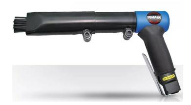
The ST-2555 pistol grip features a thermally insulated handle and a lever-style throttle for easy operation, providing an ergonomic and comfortable feel. Made from high-strength alloys, these tools are vital in the corrosion control industry as they help minimise downtime.
